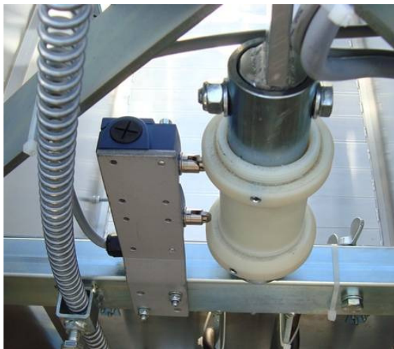
Figure 6: Overload/underload safety device
