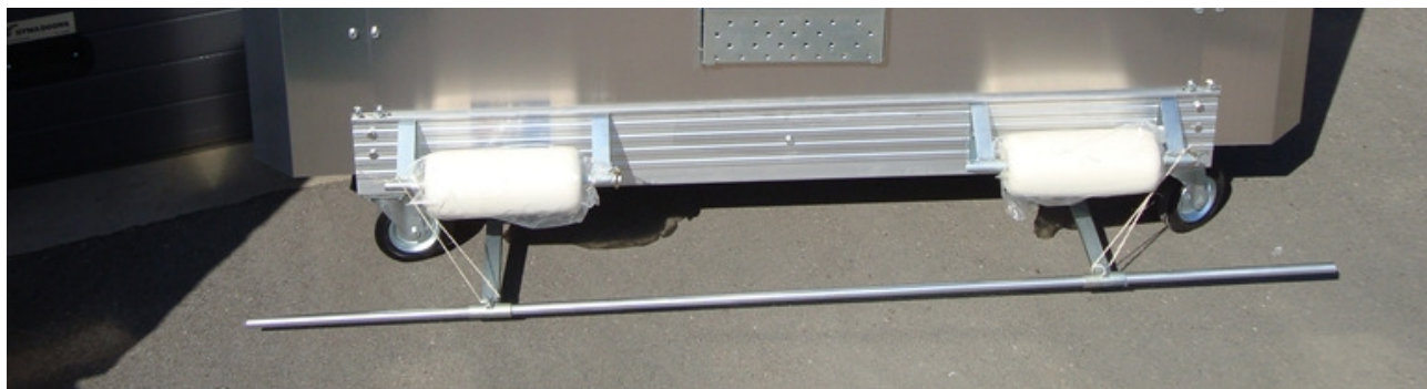
Figure 11: bottom limit trip bar and wall rollers
